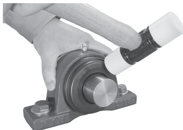
Fig. 14.12 Installing steel plate covers
