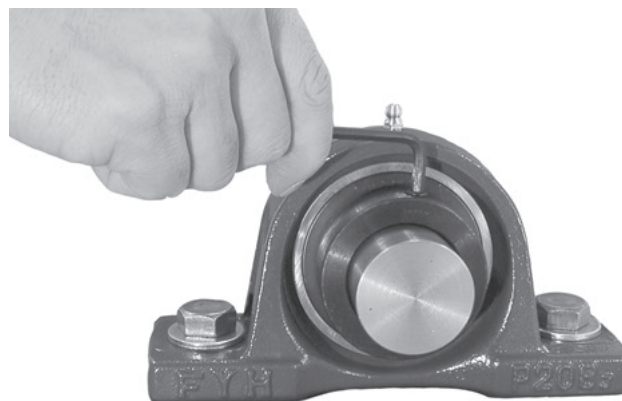
Fig. 14.10 Installing eccentric locking collar
