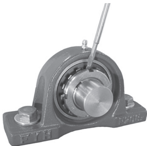
Fig. 14.8 Bending claw of washer (Locking locknut)
